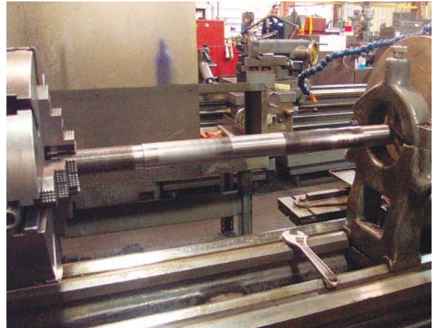
Removing old rider bands from 20" piston.
